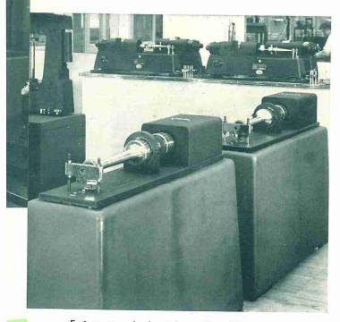
Fatigue strength of metal, as affected by composition, heat treatment and forging methods, is determined by tests conducted on a battery of fatigue testing machines of various sizes. Accurately formed test bars are subjected to fluctuating stress from 2600 to 10,000 cycles per minute through alternate compression and tension to find the endurance limit of the metal.
