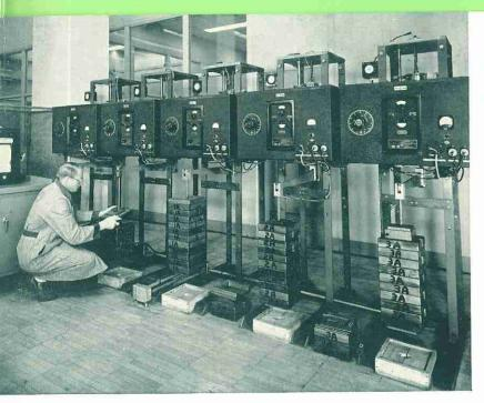
A continuing research program on the behavior of metals at elevated temperatures is facilitated in the Ladish laboratories through use of more than a score of sensitive stressrupture and creep-testing units. Test results provide a sound basis for specification of proper materials for service at elevated temperatures and verify conformity of the finished product to specifications.
