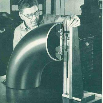
Geometric accuracy of Ladish Seamless Welding Fittings is verified by specially designed gauges.
