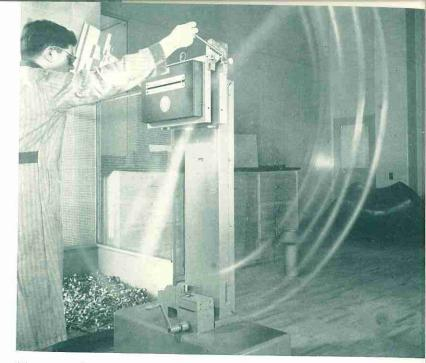
Measuring relative toughness of metal determines its ability to withstand suddenly applied impact loads. A pendulum type impact testing machine is used in the Ladish metallurgical laboratory to perform hundreds of Charpy and Izod tests daily on notched bar samples.
