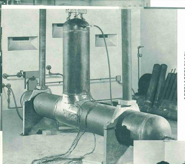
Another phase of Controlled Quality is the continuing effort of Ladish metallurgists to determine scientifically endurance limits of finished fittings. In this subterranean burst chamber, behind concrete walls, fittings are subjected to tremendous internal hydrostatic loads and external mechanical loading far in excess of the service for which they are rated. Strain measurements taken under these excessive loads help Ladish research engineers to improve designs and assure safe operation.
