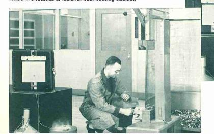
Metal's ability to stand up under severe shock and strain at temperatures far below those encountered in service is essential to fittings reliability. Impact notched bar tests in the Ladish laboratory are carried on at temperatures as low as  $-320^{\circ}$  F, to insure against brittleness under subzero operating conditions,
