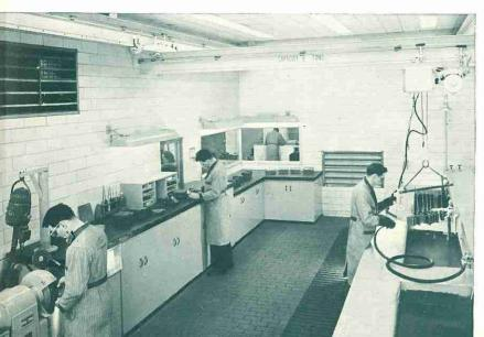
Macro-etched test sections of billets in each lot of steel provide Ladish metallurgists with data indicative of the uniformity of metal quality. Grain flow patterns of finished forgings are also checked by this method.
