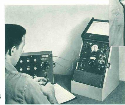
Strain gauge measurements through sensitive electronic circuits connected to stressed areas of the fittings under test provide data verifying the high safety factors built into the design of every Ladish fitting. Such scientific methods are typical of the thoroughness of Ladish research and engineering.
