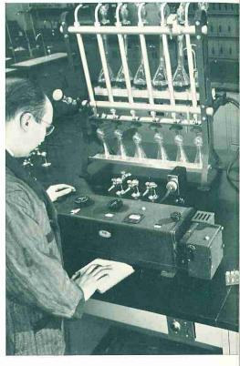
Spectrophotometry is employed in accurate determination of metal composition by measuring color intensity at various wave lengths of light transmitted through solutions of the metal under examination.
